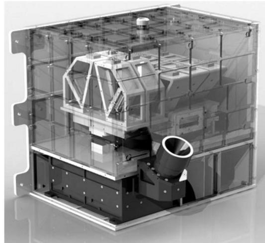
Figure 1. Overall view of the measurement block of the soft X-ray spectrophotometer ChemiX.
