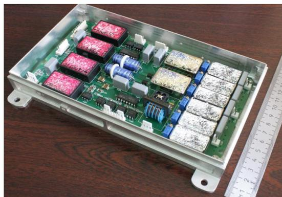
Figure 4. Overall view of the secondary supply unit
