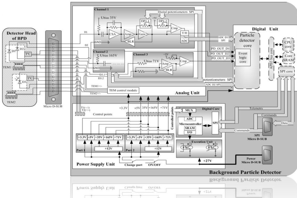
Figure 3. Block-scheme of internal electric design of the Background Particle Monitor.
