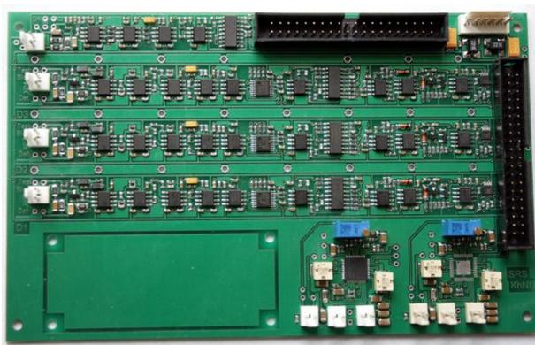
**Figure 5. General view of the printed circuit board of analog signal processing**
