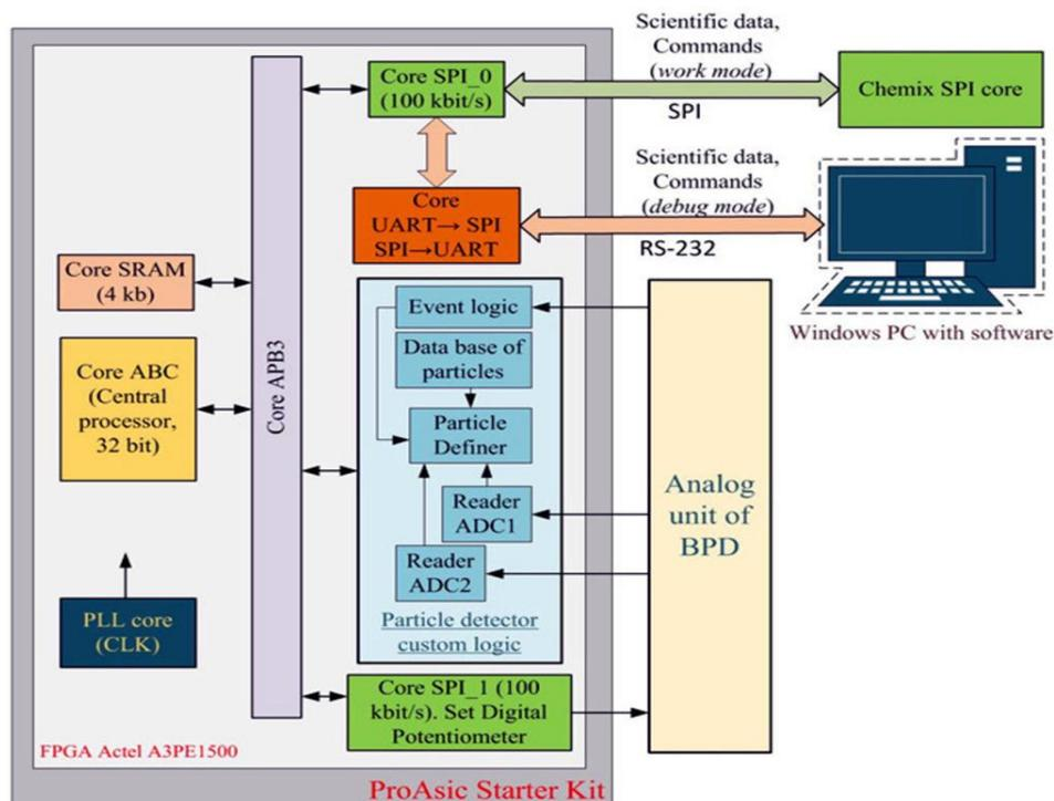
**Figure 6. Block-scheme of the Actel ProASIC3e A3PE1500 FPGA project; structure of procedure for signals exchange procedure between FPGA and the BPM's analog units and ChemiX's simulator.**
