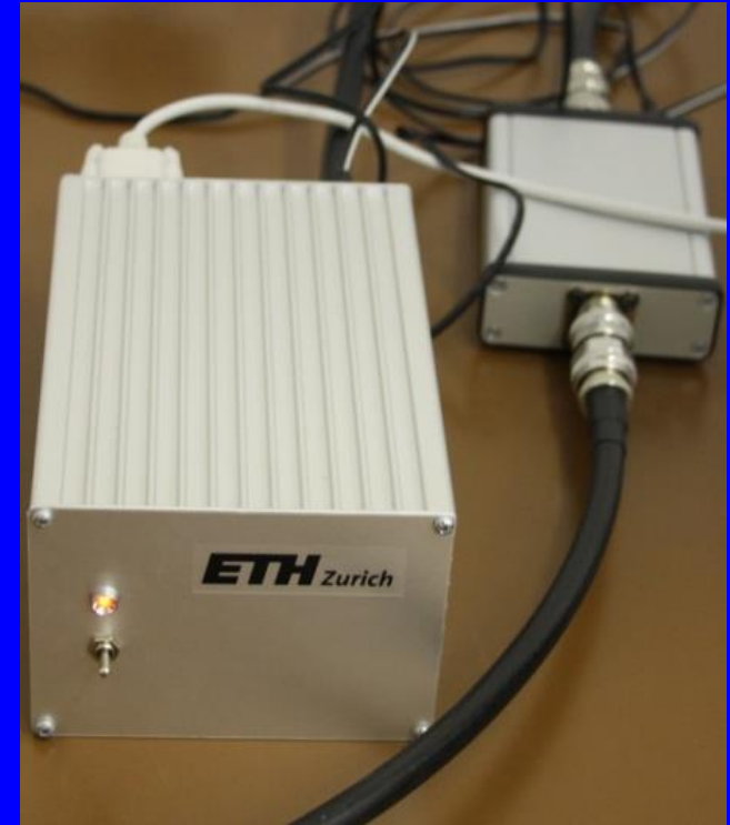
CALLISTO eC50 (left) and amplifier Frequency range: 45 – 870 MHz, Frequency resolution: 62,5 kHz
