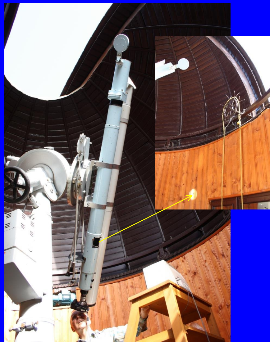
Coronagraph, observation of prominences , D /primary focus/ effective focuse - 9/125/375 cm
