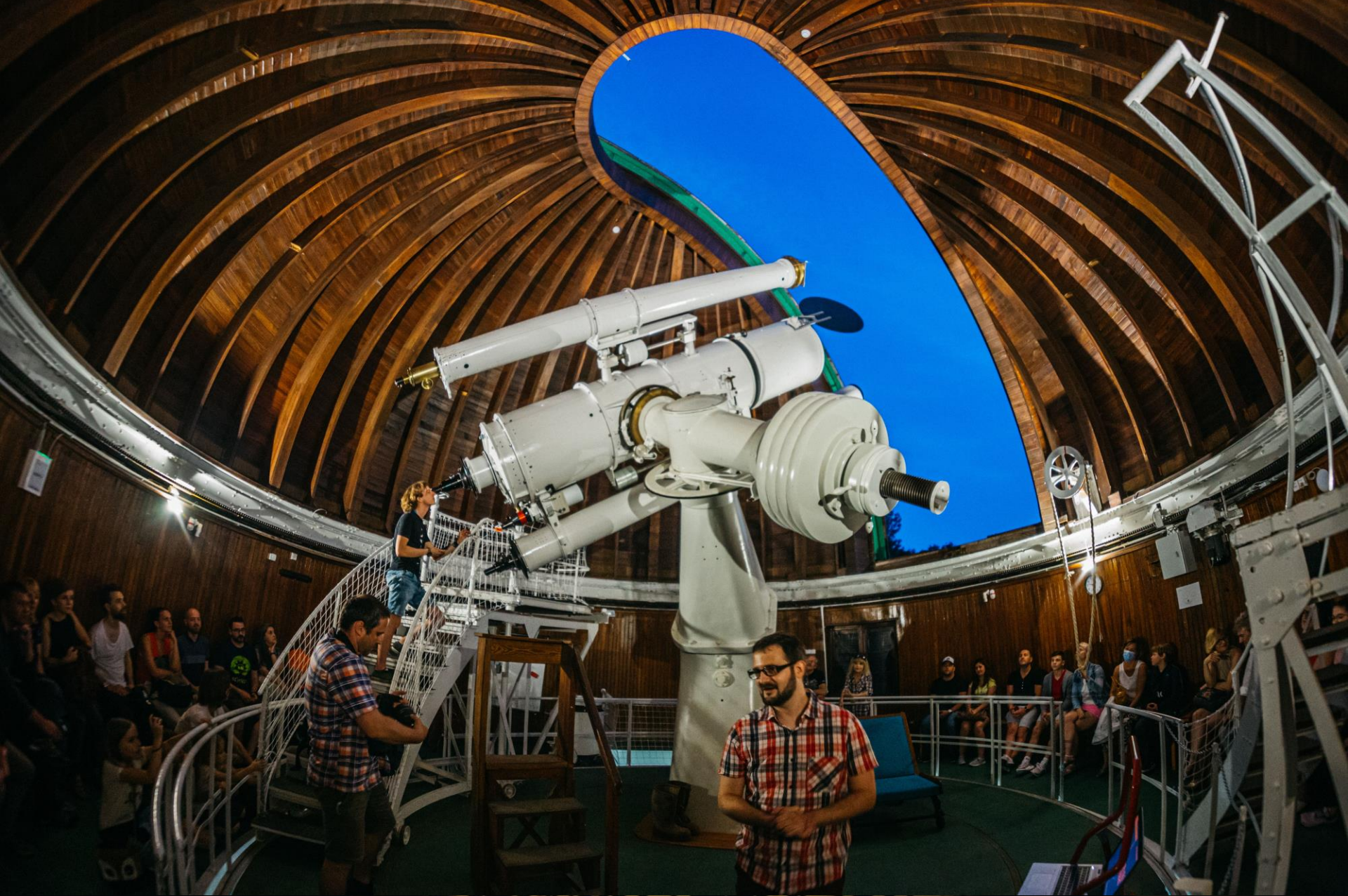
The 25-cm Merz-Konkoly refractor as a public instrument on the 60-cm telescope at Konkoly Observatory, Budapest, 2021
